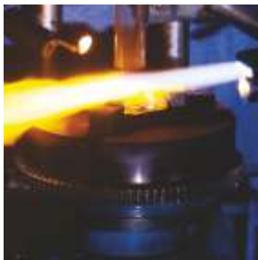
AUTOMATIC CYLINDER FORMING MACHINE : 800 pcs per shift
